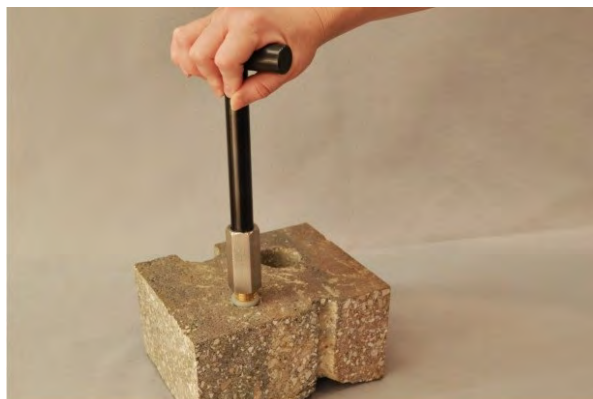
Figure 7. Removing the Vapor Pin™.
